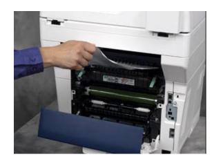
Open the rear cover to remove jams below or above the fuser
