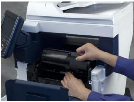
Move the Control Panel to the left, and then open the Front Door. Slide the Toner lock lever to the **unlocked** position. Push until you hear it click into the unlocked position.
