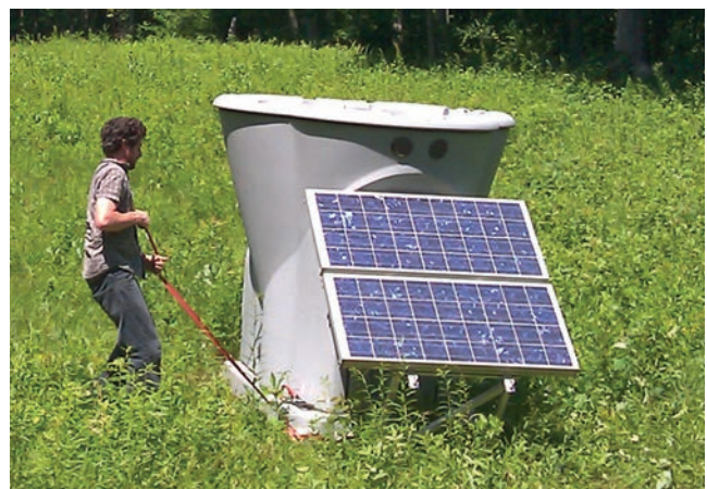
Sonic Detection And Ranging (SODAR) unit being installed
